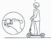
3. When the sliding of the skate starts, put the second foot to balance and press the accelerator
