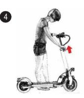
Turn the handlebar fixing lever and raise the bar to the desired position. Once raised, tighten the handle.
