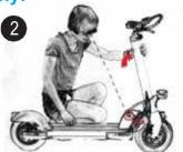
Raise the lever to fix the folding handle while firmly holding the folding bar.
