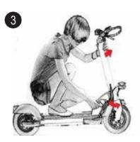
Move the handlebar bar back and forth to check that it does not move and is fixed. Check the brake drive.
