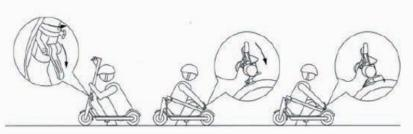
Then make sure the electric scooter is turned off and from the vertical tube take out the folding wrench, fold the tube towards the rear wheel.
