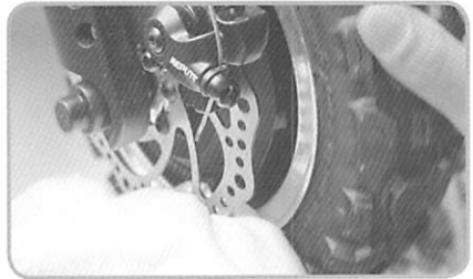
(4) Wipe the inner side of the disc while rotating the wheel.
